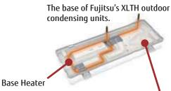
When temperatures reach 36°F, a built-in heater turns on so that any condensation doesn't freeze. Without a heater, freezing condensate can cause noise, damage to the outdoor unit and decrease system performance.
