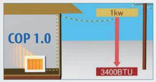
An electric heater converts electricity directly to heat. For every kW of electricity used, 3,400 BTU/h of heat are produced. Ironically, electric heaters are 100% efficient, however the ratio of power input to heat output\* is only 1.0.
