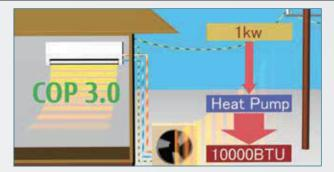
Heat pumps are more efficient than many other forms of heating because heat pumps do not actually create heat - they just move it from one place to another. For example, a heat pump with a COP of 3.0 will produce three times the heat output per power input, compared to an electric resistance heater with a COP of 1.0.
